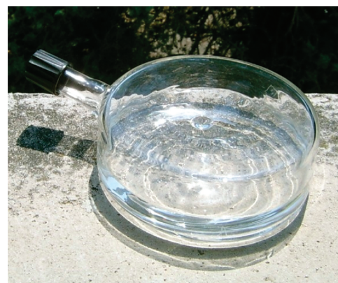
FIGURE 1. The reactions were carried out on 100 mL solution corresponding to a layer of about 1 cm thick with a surface area of about 1 dm 2 in the cylindrical Pyrex vessel used.
